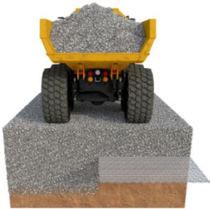
Figure 1 – Reduction in thickness with a Tensar MSL
