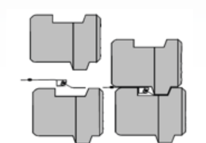
TensarTech® TW1 system provides a positive mechanical connection between the geogrid reinforcement and facing units, improving load transfer efficiency, connection integrity, and the long-term structural performance of the reinforced soil structure
