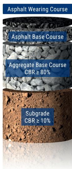
Conforming Non-stabilised Section
