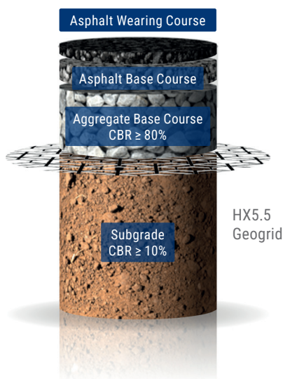
Tensar Stabilised Section
